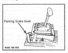
To apply parking brake, press emergency/parking brake pedal, push the parking brake lever foreward then release pedal. Press and release brake pedal to disengage parking brake.
