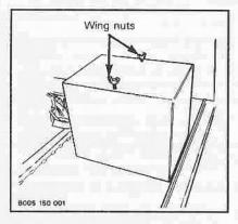
Check electrolyte level in each cell. Add distilled water if necessary.
