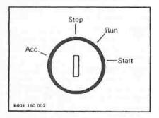
To stop the engine; turn ignition key to STOP position.
