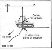
This could compare to the action of a seesaw with the vertical line forming the center or pivot of the seesaw. When more weight is placed on one side than the other, the seesaw will move in that direction.
