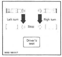
Steering is by means of the steering levers. Pulling on one lever applies the corresponding brake band on one drum of the differential. This slows the axle gear on that side and increases the speed of the axle gear on the other side. One track running faster than the other makes the vehicle turn. This type of differential, provides traction to both tracks, even when turning.
