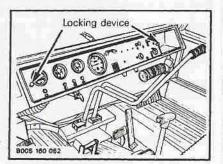
To remove instrument panel; push and turn locking device a quarter turn.
