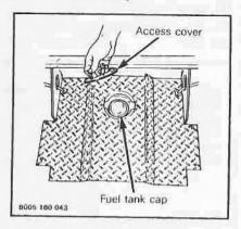
To gain access to the fuel tank cap, remove the access cover which is located behind the engine hood.
