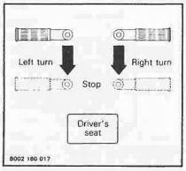
To steer the vehicle in a give direction, pull the lever corresponding to that direction.
