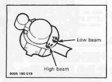
The dimmer switch, located on left steering lever, allows selection of high or low headlamp beam. To select high or low beam flick switch.
