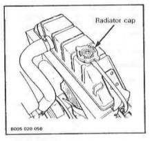
Always check coolant level when engine is cold.
