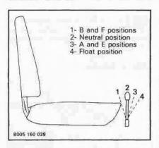
NOTE: When not engaged in float position, the levers normally return to neutral position.
