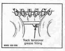
Tracks are adjusted by means of hydraulic track tensioners located between the two rear wheels. To tighten tracks, inject grease through grease fitting on track tensioner. To loosen tracks, bleed track tensioner by means of the bleeder tool.
