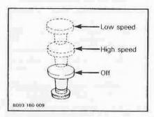
Controls the heater/defroster fan speed.
