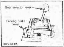
To apply parking brake, depress the emergency/parking brake pedal and push the parking brake lever foreward then release pedal. Depress pedal and release to disengage parking brake.
