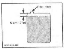
Coolant level must 5 cm (2 in) below bottom of filler neck.
