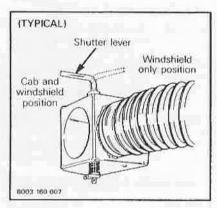
NOTE: A manually-operated shutter located over the left footrest can be activated to send hot air to the cab and/or the windshield.
