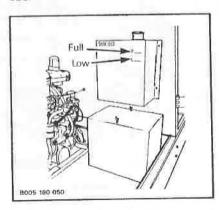
Differential Oil Level At room temperature (21°C (70°F) approx.)), the oil level should reach line "F" on the tank.
