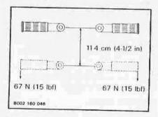
Both steering levers should have a travel of approximately 11.4 cm (4-1/2 in) when a force of 67 N (15 lbf) is applied at each handle.
