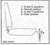
NOTE: When not engaged in float position the lever normally returns to neutral position.
